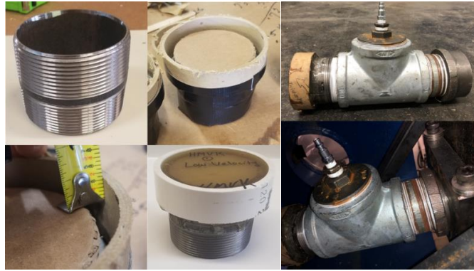
Figure 1. Single wall self-sealing studies test configuration. Each of the 12 selected elastomers were bonded to a 7.62 cm NPT coupler and mounted to the pressurized tank system presented.
