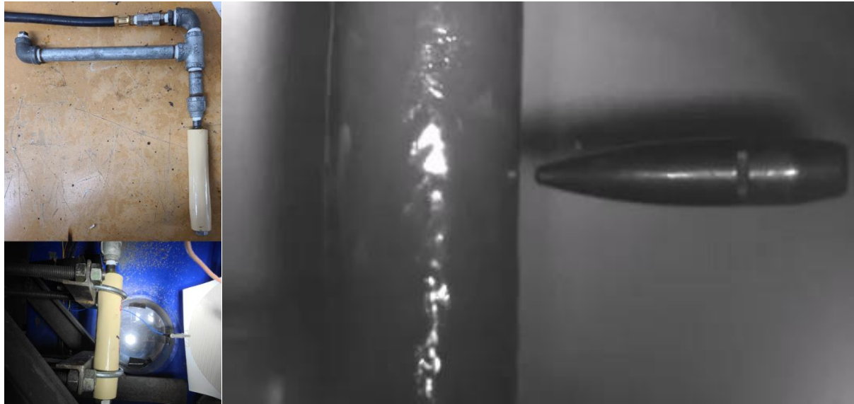
Figure 2. Self-sealing hose system test fixture. For both homogeneous and heterogeneous self-sealing studies. The mounting system enables alignment of the hose center to the flight path of the projectile.
